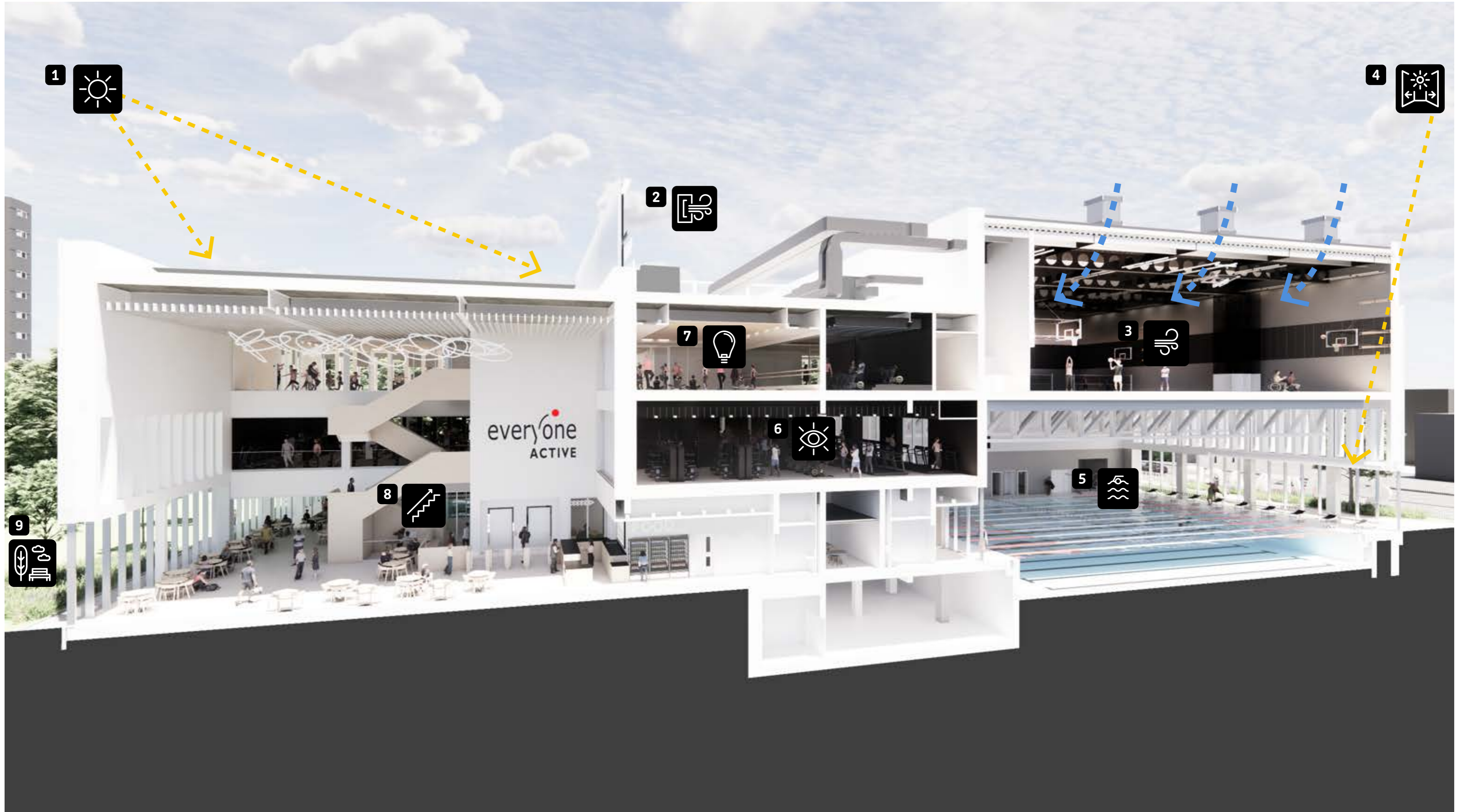
Building in section showing sustainability features
