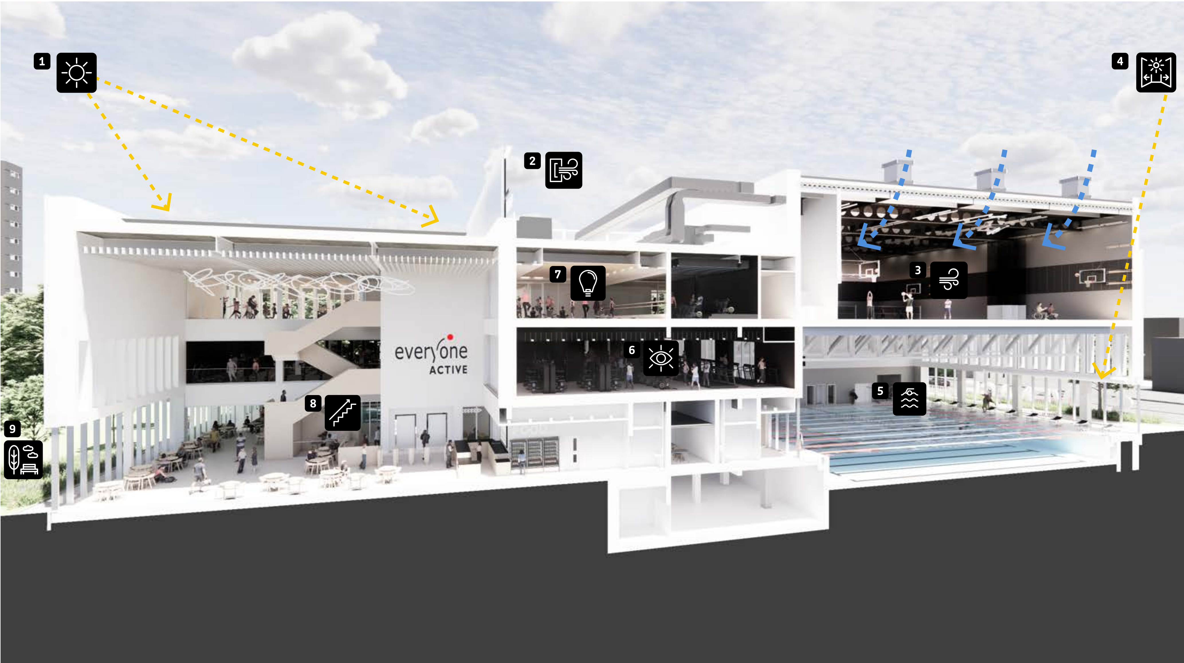
Building in section showing sustainability features
